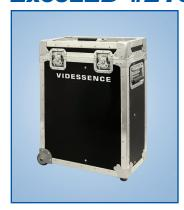
Heavy-duty flight case for the ExceLED #E100 is made of fiberglass laminate, internally framed with light metal and has metal corner braces and framing. Dense foam lining protects fixture in airline and overland transport. Recessed, spring loaded handles are provided for lifting and handling. Recessed casters for rolling. #CS-E100-FC
