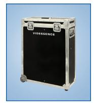
Heavy-duty flight case for the ExceLED #E225 is made of fiberglass laminate, internally framed with light metal and has metal corner braces and framing. Dense foam lining protects fixture in airline and overland transport. Recessed, spring loaded handles are provided for lifting and handling. Recessed casters for rolling. #CS-E225-FC
