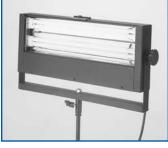
This is a versatile, short throw location lighting fixture. It is small and easy to handle or mount in tight quarters. The.063 formed aluminum housing has a textured black TGIC polyester powder coat finish. It utilizes two 55 watt Fluorescent Biax lamps. The fixture produces an equivalent
