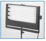
This is a powerful, high output location lighting fixture. The .063 formed aluminum housing has a textured black TGIC polyester powder coat finish. It utilizes four 55 watt Fluorescent Biax lamps and each pair can be separately switched. In full "on" this fixture produces an equivalent
